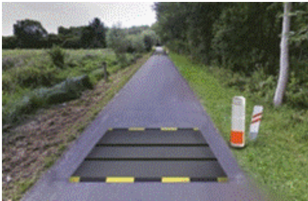
Figure 14 - Speed bumps and flashing posts
