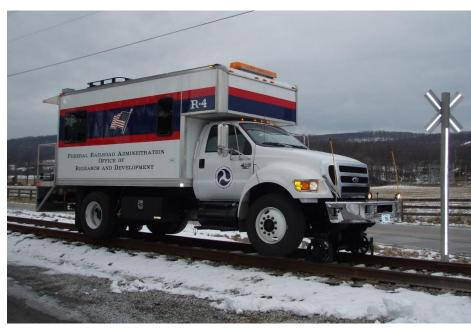
LiDAR Surveying System to be installed on the Hi-Rail "R4" research vehicle.
