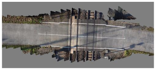
Figure 16: Example of LC photogrammetric model (source: SNCF)
