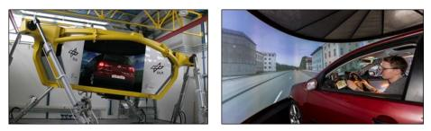
Figure 4: DynSim (Dynamic Driving Simulator)
