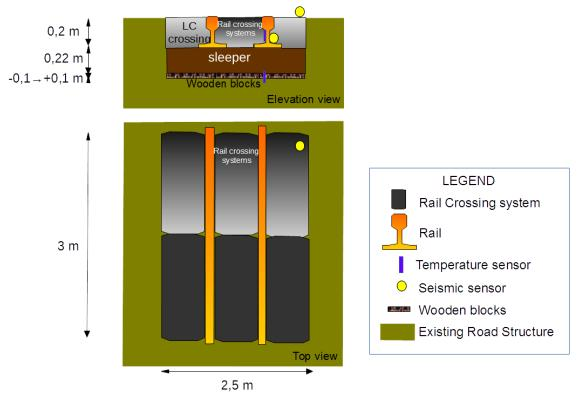
Figure 13: Experimental structure with instrumentation
