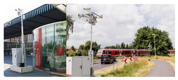
Figure 26: Mobile sensor poles at railway station and level crossing
