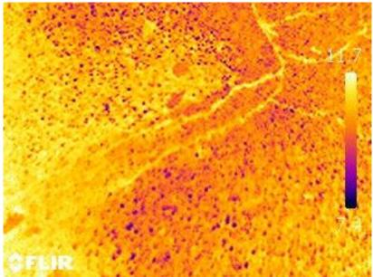
**Figure 18:** Thermal infrared observation of thin fractures on a road during afternoon in winter. Note the temperature contrast between the fractures and the surrounding medium
