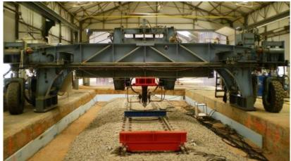
Figure 10: A hydraulic jack fixed in a loading gantry
