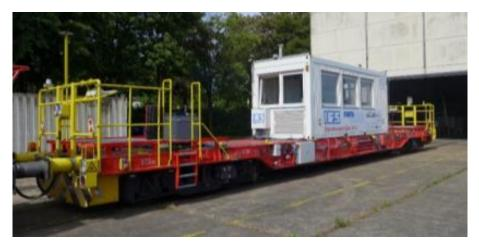
Figure 8: Testing rail vehicle
