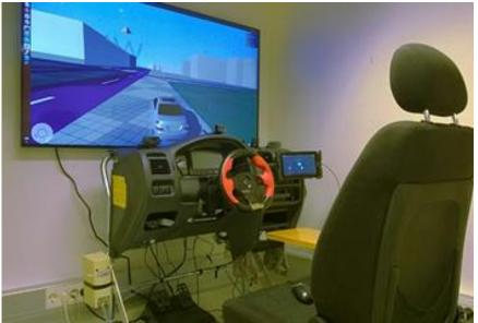
Figure 24: Simulation environment for ITS application testing and development. © VTT
