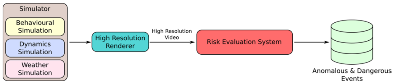
Figure 10: Overview of the complete architecture using the video synthesis system as input of the risk evaluation system.
