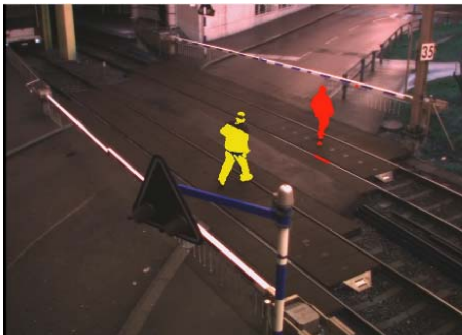
Figure 21: Two pedestrians clearly detected when crossing the LC.
