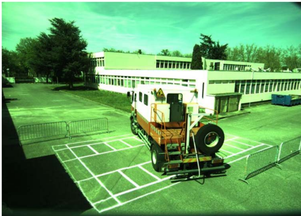
Figure 7: Mockup level crossing installed at Cerema Toulouse. A big truck zigzagging while the barriers are closed.
