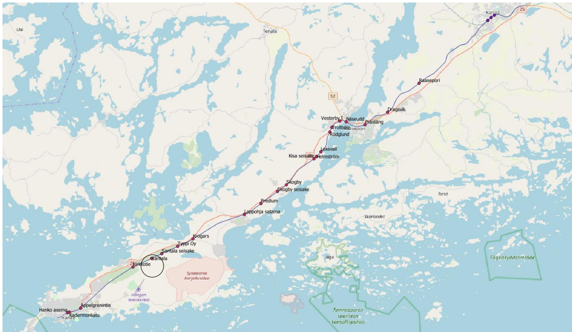
Figure 10. Rail section 142 and its level crossings. Red circle means protected LC, green is unprotected, blue circle is a station.
