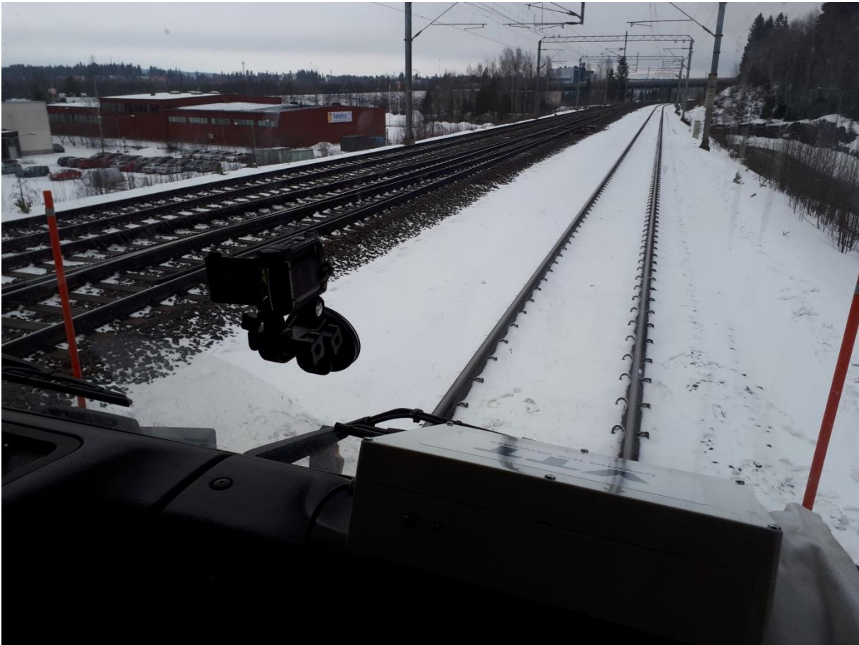
Figure 49. A view from the cockpit. An action camera has been installed directly to the wind screen.
