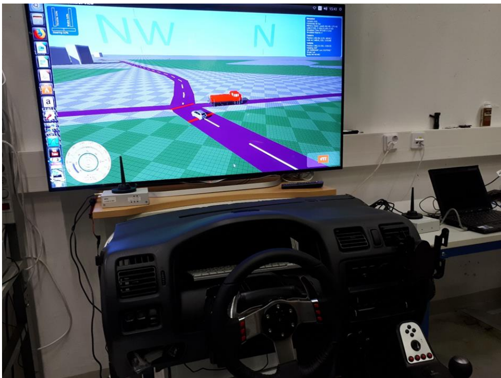
Figure 14. Picture of road traffic simulator view.
