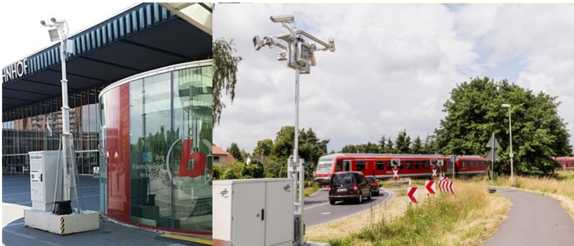
Figure 53. MTD sensor poles at a railway station and a level crossing (not identical to test site).
