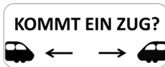
Figure 3. Sign used to indicate safe behavior for road users at passive level crossings asking the road user to check whether a train is approaching.
