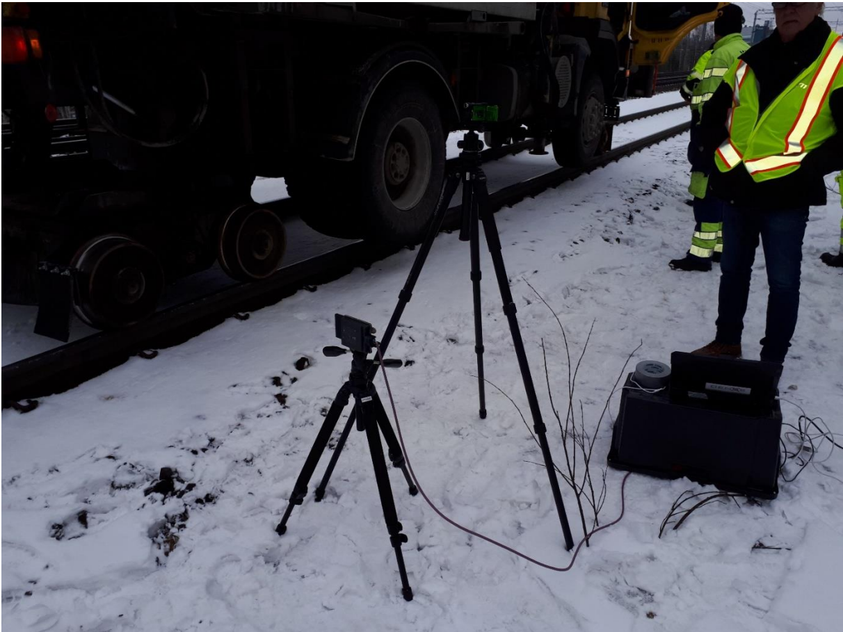
Figure 48. Camera and the radar have been installed on tripods.
