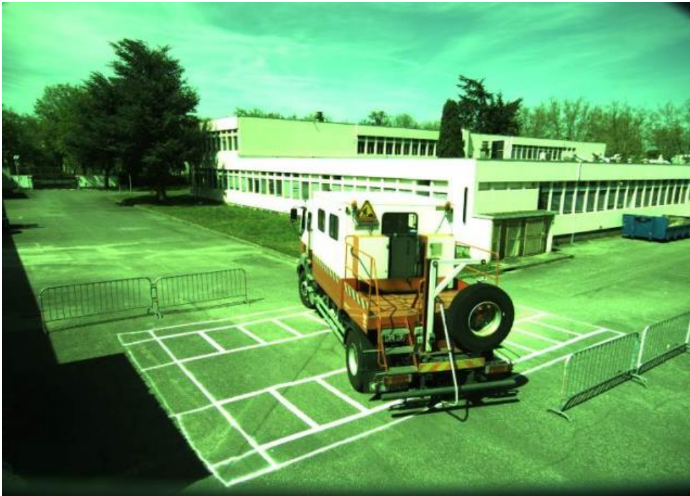
Photo 7: Mockup of a level crossing installed at Cerema Toulouse a big truck zigzagging while the barriers are closed.
