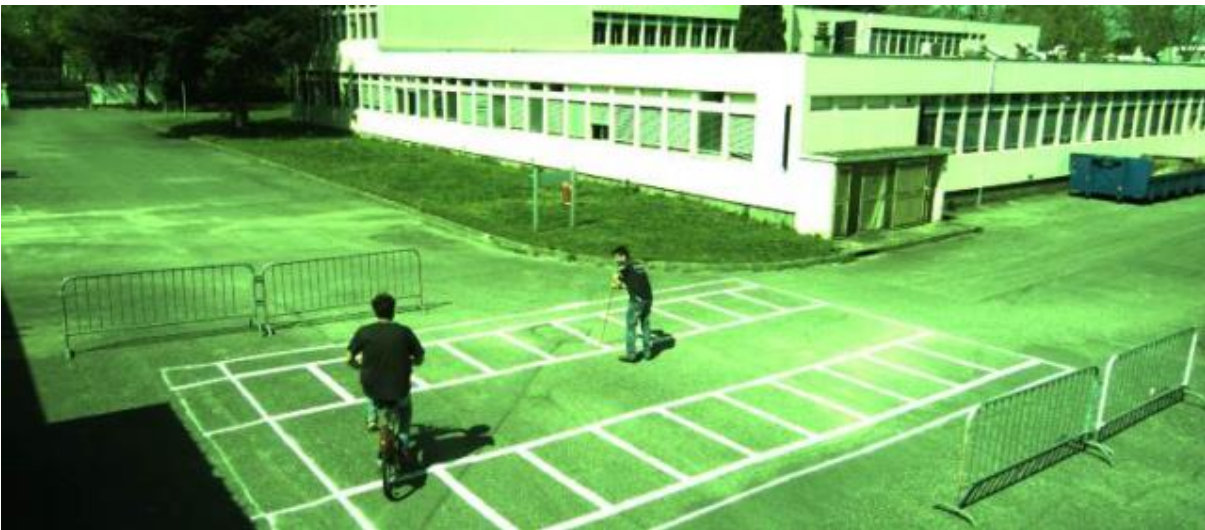
Photo 6: Mockup of a level crossing installed at Cerema Toulouse with a pedestrian and bicycle crossing the LC at the same time
