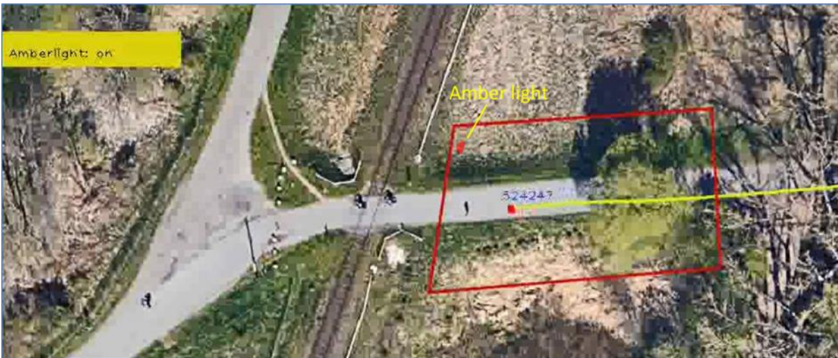
Figure A9. Geofencing for triggering the blinking of the amber light (see text for procedure).
