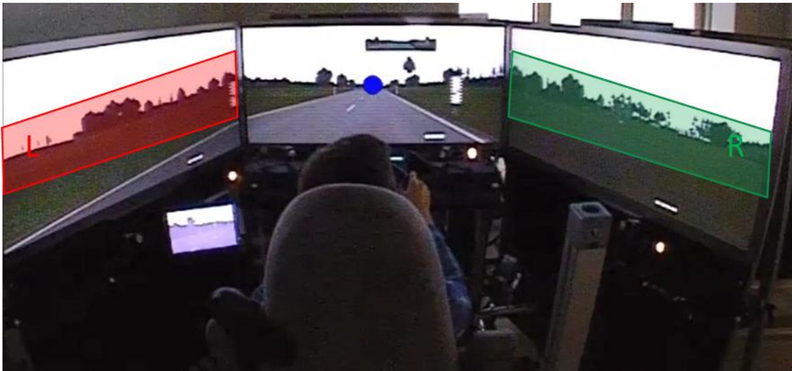
Figure 3. Definition of the regions of interest (ROI) “left periphery” (L) and “right periphery” (R). The blue dot represents the participant’s current gaze position in this screenshot.
