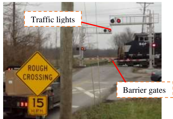
Figure 3. Level crossing with Strail material and approaching road (left), active level crossing with traffic lights and barrier gates (right).
