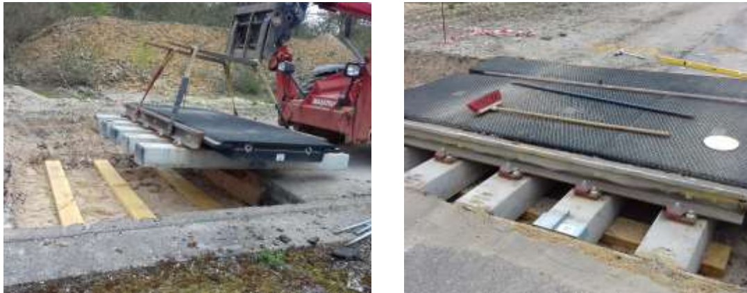
Figure 14. Configuration 1 – Bump with wood beams
