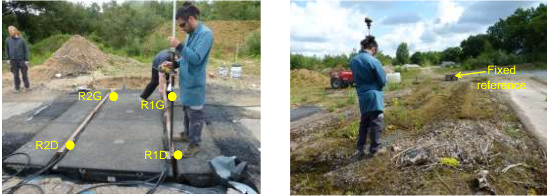
Figure 31 : Rail leveling and reference measure of the full station.
