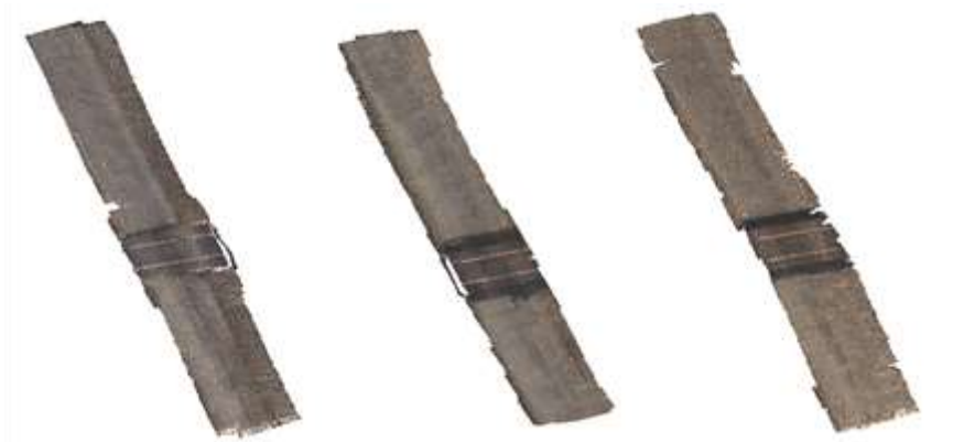
Figure 57. Photogrammetric model – Bump configuration (left to right 0, 3.5 and 7 cm).
