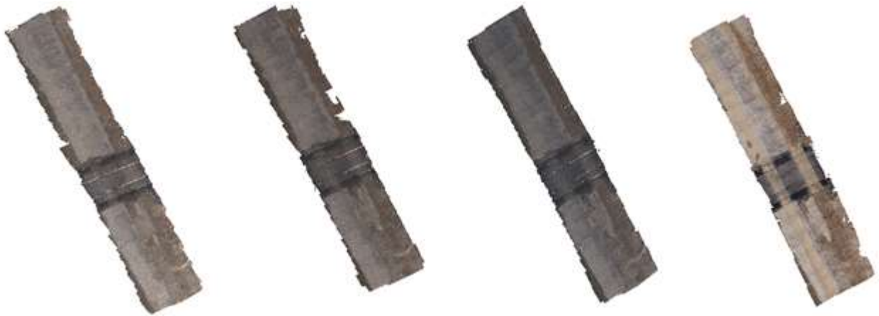
Figure 58. Photogrammetric model – Hollow configuration (left to right 0, 3, 5 and 5.7 cm).
